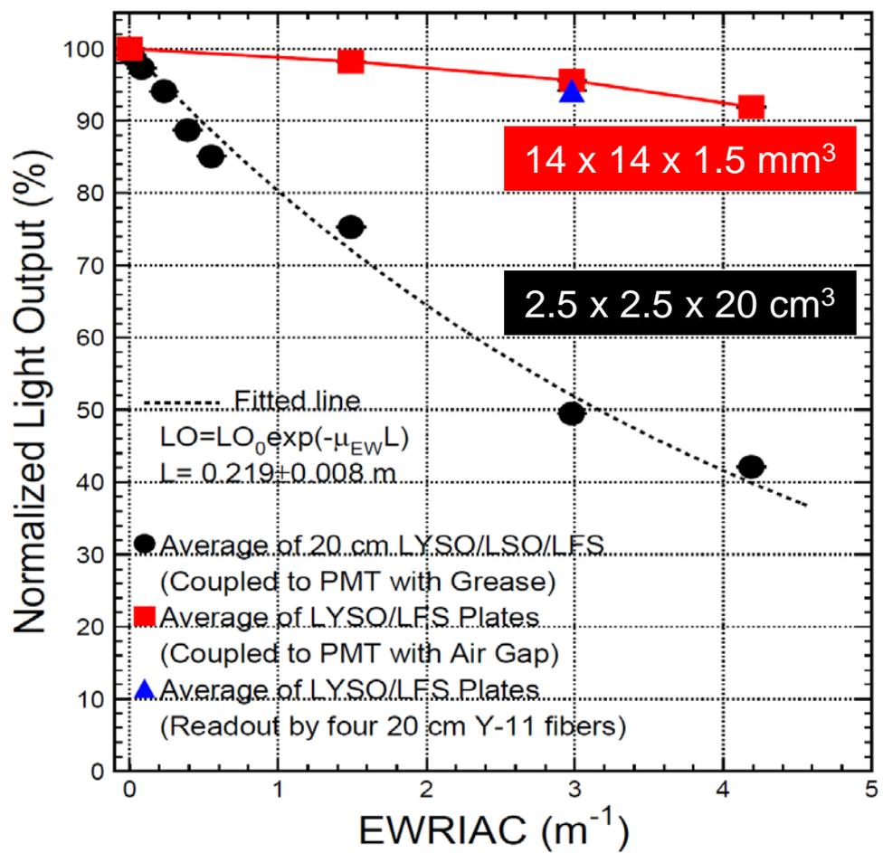
LO loss of LYSO plates after 100 Mrad is 4%/6% for direct/WLS readout
