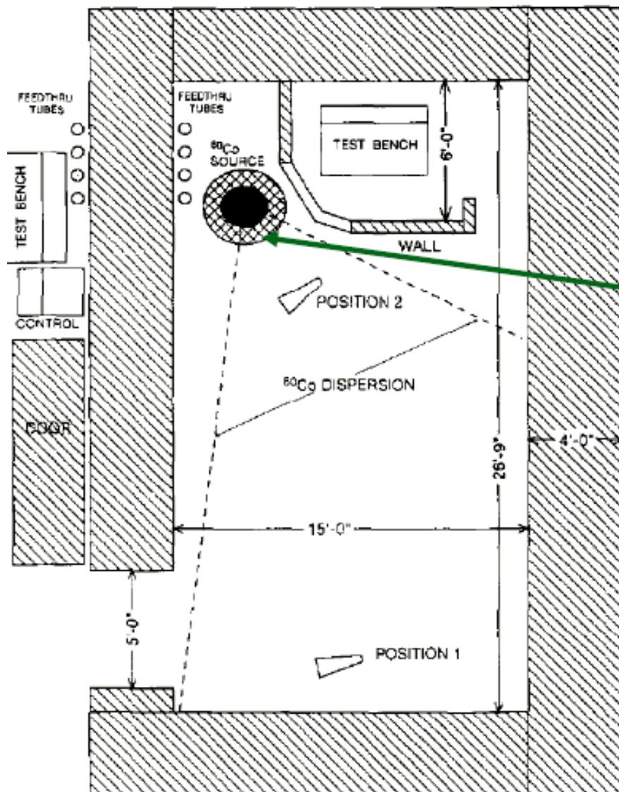
Two high intensity  $^{60}\text{Co}$  sources provide variable dose rates up to 1 Mrad/h in an opening throat of 10" x 10" x 13.5".
